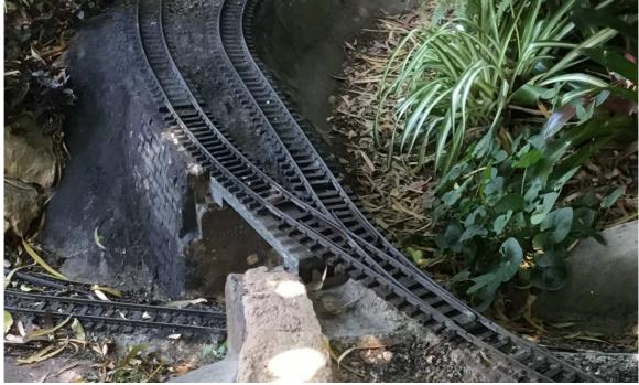
The present arrangement shows the right hand turnout points partially "on the bridge".
